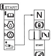
Check the engine's oil level Check the hydrostat's oil level Lift up the cutting unit Put the gear shift/hydrostat pedal in neutral Brake If the engine is cold use the choke Start the engine Release the parking brake before
